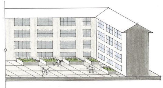
Flow-through planters on the plaza level of a podium-style development.
