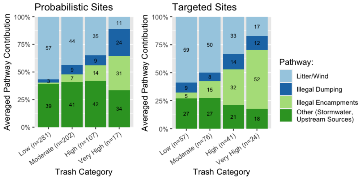
Figure 4-14. Average contributions of trash observed from each pathway to probabilistic and targeted receiving water monitoring sites during monitoring events. Monitoring events are grouped by trash condition categories.
