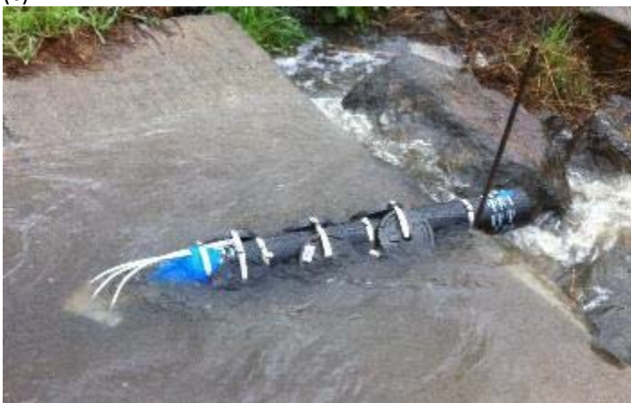
Figure 2. Sampling equipment used in the field. (a) Painter's pole, Teflon tubing and an ISCO used as a slave pump; (b) Teflon bottle attached to the end of a DH81 sampling pole; (c) a Walling Tube suspended sediment sampler secured by 5-lb weights along the body of the tube (because it is sitting atop a concrete bed) and rebar driven into the natural bed at the back of the sampler.
