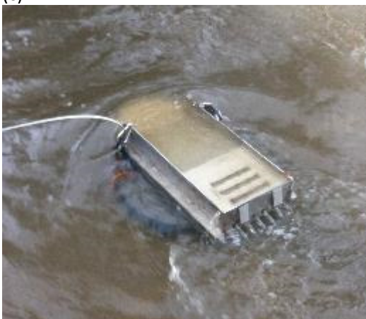
Figure 2. Sampling equipment used in the field. (a) Painter's pole, Teflon tubing, and an ISCO used as a slave pump; (b) Teflon bottle attached to the end of a DH81 sampling pole; (c) a Hamlin suspended sediment sampler secured atop a 45-lb plate; and (d) a Walling Tube suspended sediment sampler secured by 5-lb weights along the body of the tube (because it is sitting atop a concrete bed) and rebar driven into the natural bed at the back of the sampler.
