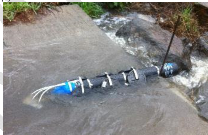
Figure 2. Sampling equipment used in the field. (a) Painter's pole, Teflon tubing, and an ISCO used as a slave pump; (b) Teflon bottle attached to the end of a DH81 sampling pole; (c) a Hamlin suspended sediment sampler secured atop a 45-lb plate; and (d) a Walling Tube suspended sediment sampler secured by 5-lb weights along the body of the tube (because it is sitting atop a concrete bed) and rebar driven into the natural bed at the back of the sampler.
