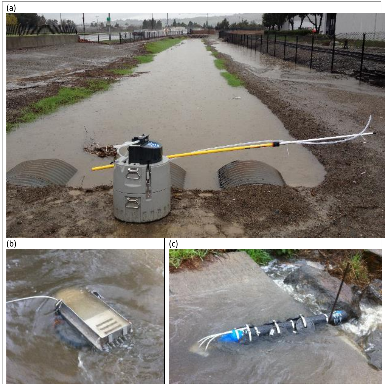
378 Figure 2. Sampling equipment used in the field. (a) Painters pole, Teflon tubing and an ISCO used as a 379 slave pump; alternatively a Teflon bottle is attached to the end of a painters pole (DH84) and used for 380 sample water collection as opposed to using an ISCO as a pump (b) Hamlin suspended sediment 381 sampler; and (c) the Walling tube suspended sediment sampler.
