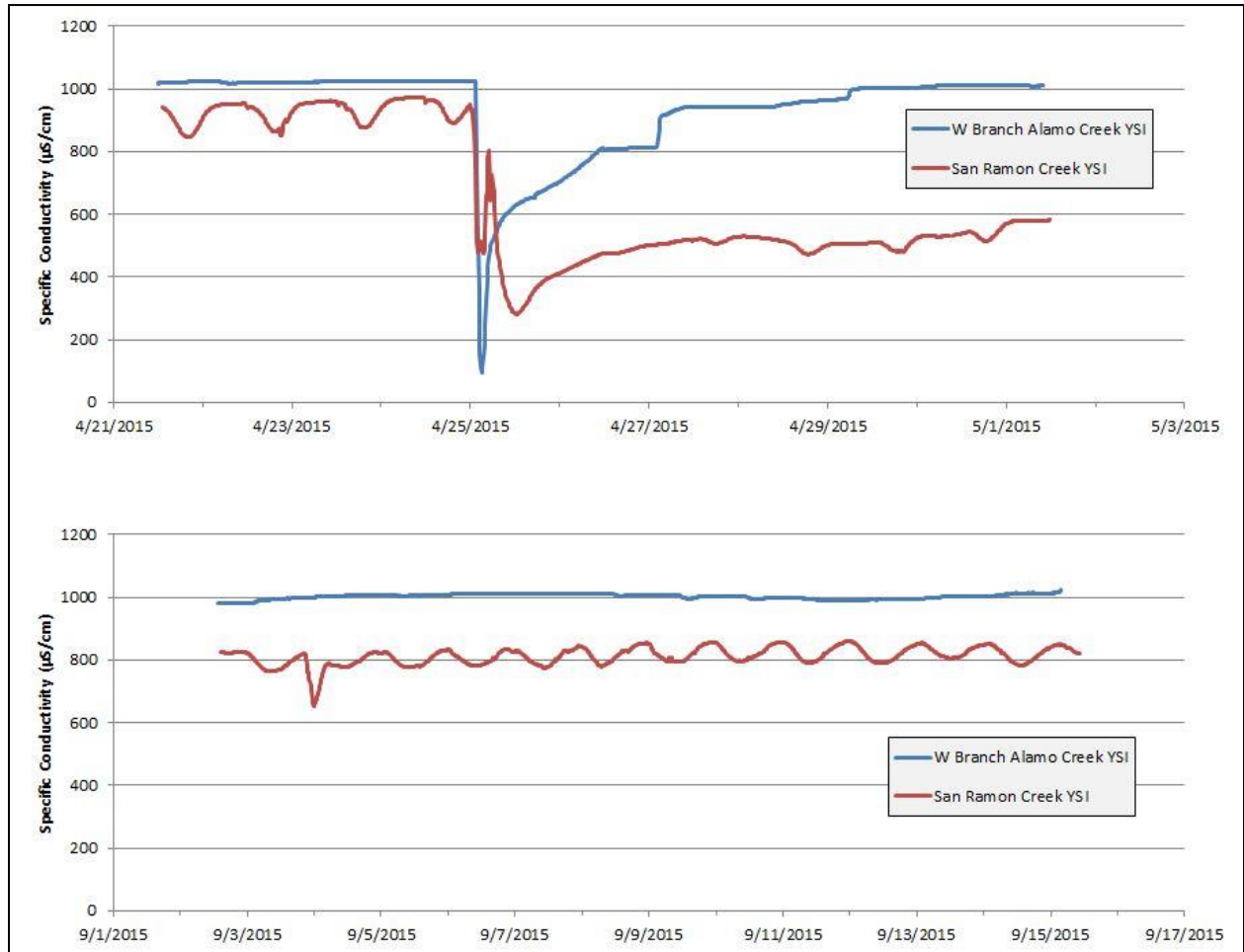
Figure 4.7 General Water Quality Data (Continuous Specific Conductivity) Collected in Contra Costa County (West Branch of Alamo Creek and San Ramon Creek), April 21-May 1 and September 2-15
