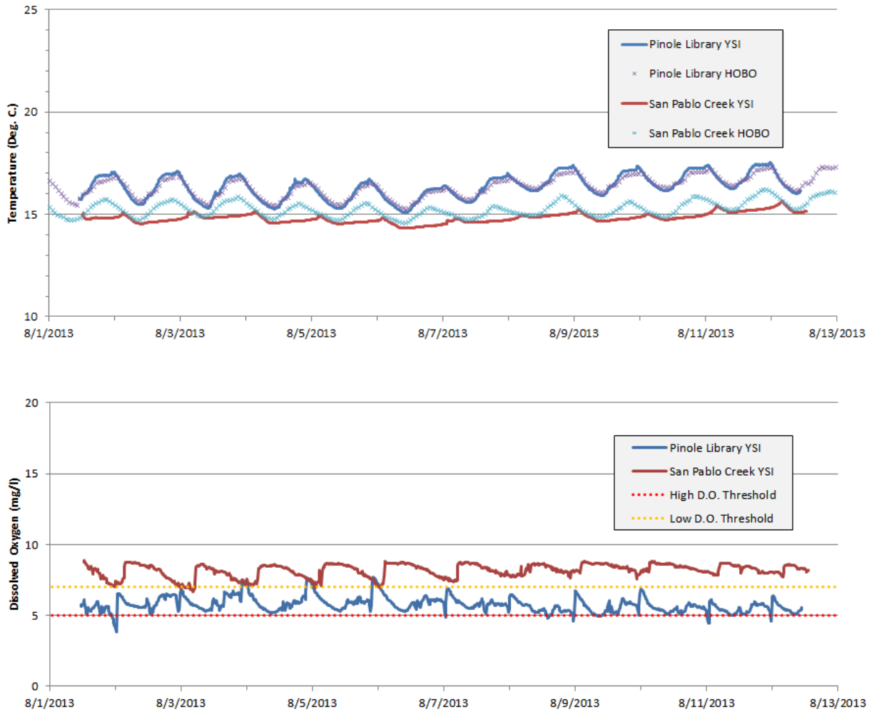
Figure 4.11a Continuous water quality data (temperature, dissolved oxygen, pH, and specific conductivity) collected at Pinole Library and San Pablo Creeks, August 1-12, 2013
