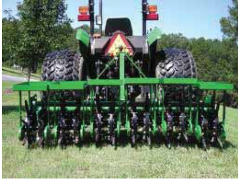
Pull-behind, cam-driven aerator
