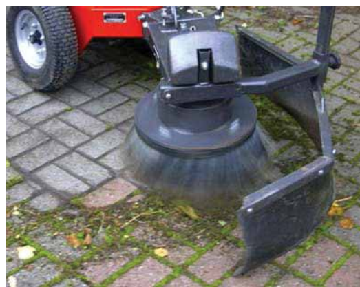
Motor-driven Weed Brush (Kersten WeedBrush®)
