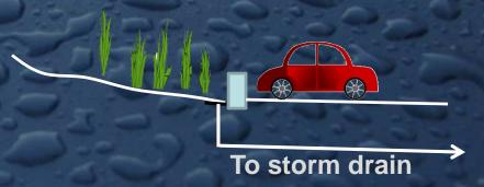
Grade self-retaining areas to drain inward. Set any area drains to pond 3"-4"
