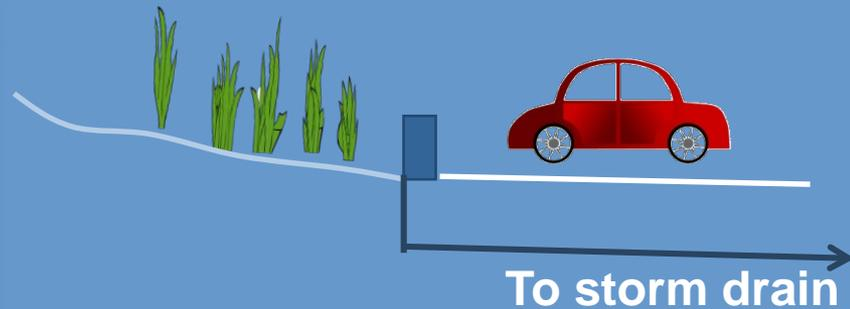
Grade self-retaining areas to drain inward. Set any area drains to pond 3"-4"
