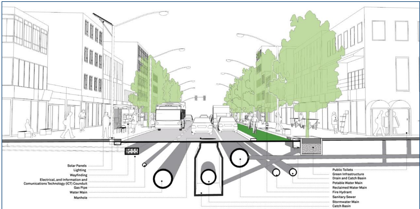
Figure 3.8. Types of underground utilities that may be encountered when siting high-flow capacity FTC systems public streets/roadways (Image courtesy of Global Designing Cities Initiative Global Street Design Guide).
