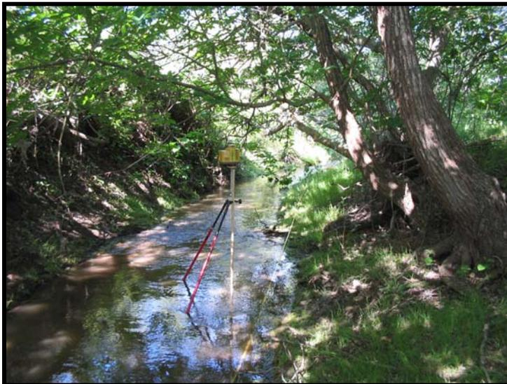
**SITE NOTES:** Stable pool-riffle channel with gravel riffles and well developed riparian corridor. High root strength in banks, moderate sinuosity. Incised slightly into valley floor. Limited inset floodplain development.
