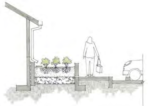
Bioretention facility adjacent to building. An impermeable cutoff wall between the facility and the building may be incorporated.
